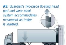
Guardian is the ideal solution for air-ride suspension trailers, which can move up and down as much as 8" during loading/unloading.
