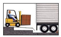
▲ Trailer Walk: During loading or unloading, the displacement of weight by the forklift can cause air-ride suspension trailers to move in an elliptical fashion, causing it to "walk" away from the dock in a more prominent motion.
