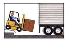
▲ Premature Departure: Truck drivers think loading is complete, or simply connect the wrong trailer and pull away while the dock attendant is still loading or unloading.
