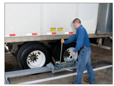
The operator slides the restraint carriage on the guide rail, positions it in front of the wheel, and pivots the restraining arm to lock it in place and secure the wheel.
