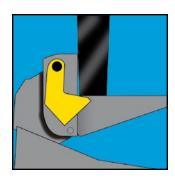
◆ The Serco system's primary locking position provides a captive reach up to 11" to engage wide, recessed or bent rear impact guards and limits trailer movement.
