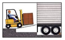
▲ Trailer Creep: Constant impact of start/stop action of a fully loaded forklift can cause the trailer to creep forward inch by inch, beyond the reach of the leveler lip, causing the leveler to slip off the back of the trailer and drop suddenly.
