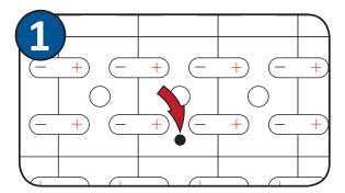
Choose probe location near the center of the battery. Drill ½" diameter hole in the cell cover with approved drill bit. Make sure there is clearance down to the plates and around the probe before drilling.
