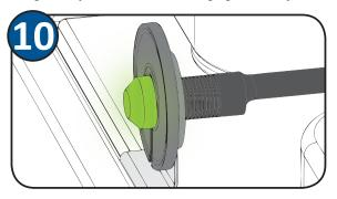
Pull the light back through the center of the large washer and push the small washer over the back of the light assembly to secure the light to the bracket.
