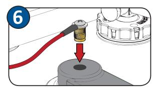
Remove the shroud and using a #2 drill bit, pre-drill a hole, 3/8" deep in the center of the post. Tap the bushing, screw and terminal into the hole with a hammer.
