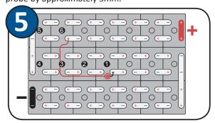
Select cell post locations for wire installation. This will require 6 cells in series with the black wire attached to the negative terminal into which the sensor is installed and the red wire attached to the positive terminal six cells up. NOTE: The wires should not be pulled tight.
