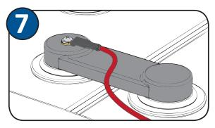
Tighten the screw. Note: Ring terminal should face down with the wire exiting at the middle of the intercell connector as shown. Apply grease to connection after securing to battery and reinstall shroud without pinching wire.
