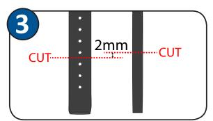
Count the same number of holes on the gauge guard starting from the bottom and cut the gauge guard at this height. Cut the sensor probe 2mm shorter than the gauge guard, then strip the heat shrink of the probe by approximately 5mm.
