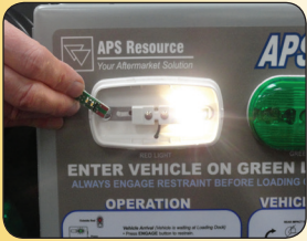
Inside LED Upgrade
